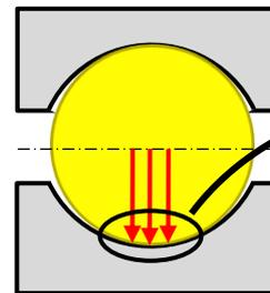
Nano Diamond on the rolling contact surface, along the slip Schematic diagram that circulates and relieves shear stress \*\*\*
