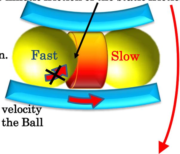
It falls into slipping that cannot be controlled because the static friction of the retainer is larger than the kinetic friction of race.
