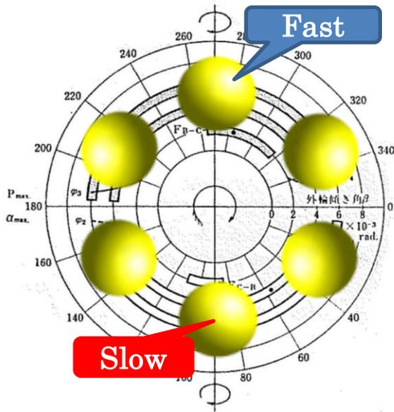
Friction increases so that slipping respect of Ball and the retainer may take the place from the kinetic friction of the static friction.
