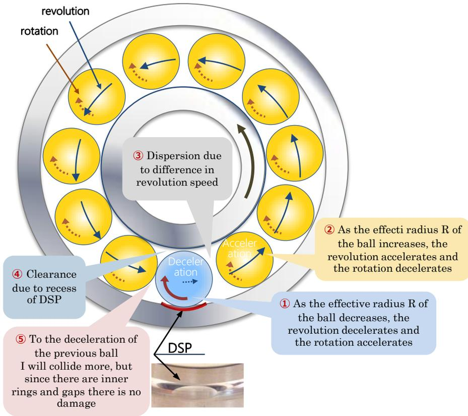
In place of the cage, ADB has one to several Dispersion Starting Points (DSP recesses) on the outer ring. By moving the contact point between the ball and the outer ring [○ in the figure] from the groove bottom of the outer ring to the two recesses of the recess, the effective radius  $R$  of the ball is decreased (see the figure below). This decrease in  $R$  will change the ratio of ball self-revolution (left figure).
