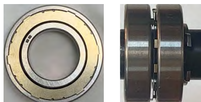
Wave washer for locking onto outer ring, for 7901 (Preload 3N, Mounting thickness 0.7mm, DB combination)
